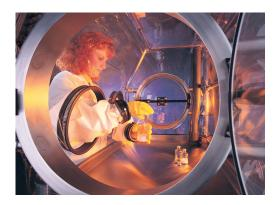
**Glovebox applications** – where materials processing and experiments must be carefully controlled and performed under low oxygen conditions - for example in bioresearch or nuclear applications.
